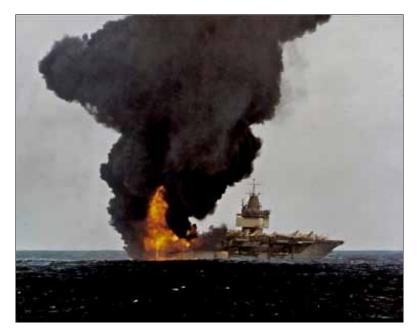
wind over the deck could be used to carry smoke and flames out aft of the ship. The only problem was that the associated list to starboard led burning fuel to track over towards the four A-7s on the starboard side of fly-3.
