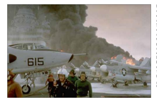
Nowhere on deck was safe from bomb explosions, fireballs, and shooting missiles. Shrapnel injured many crew, damaged many aircraft and peppered the island superstructure, penetrating the SPS-32 and -33 panels and embedding in an ECM Dipole aerial on the beehive. Planes were moved forward to Fly 1 and Fly 2 to create a fire-break.
