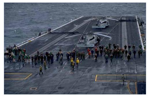
The first FOD walk-down of Big E's flight deck for the 1998–1999 deployment – a twice-daily ritual. The crew are searching the recently laid and painted non-skid deck for debris that could become ingested by and damage aircraft engines. Centurion status on *Enterprise* was awarded not only to pilots for landing 100 times, but also to those who regularly attend the FOD walk-down.
