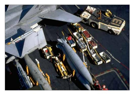
An MD-3D "mule" sits amid ordnance, drop tanks, an ALQ-99 jamming pod, and a VMFA-312 Hornet in the "bomb farm" area aft of the superstructure. Note that mule 13 had the standard turbine attached, making it a "Huffer cart." In the right foreground is an ordnance elevator hatch, outlined in the usual yellow- and red-dashed line.
