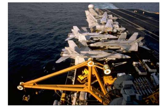
Painted brilliant yellow in 1998 the aircraft crash crane sits as out of the way as possible behind the island. In the event of mishap resulting in a stricken aircraft blocking the deck, Tilly would lift the crippled bird away. In the foreground is one of the two antennas for the AN/SPN-46 used in the PALS by CATCC-65 to assist pilots aboard.
