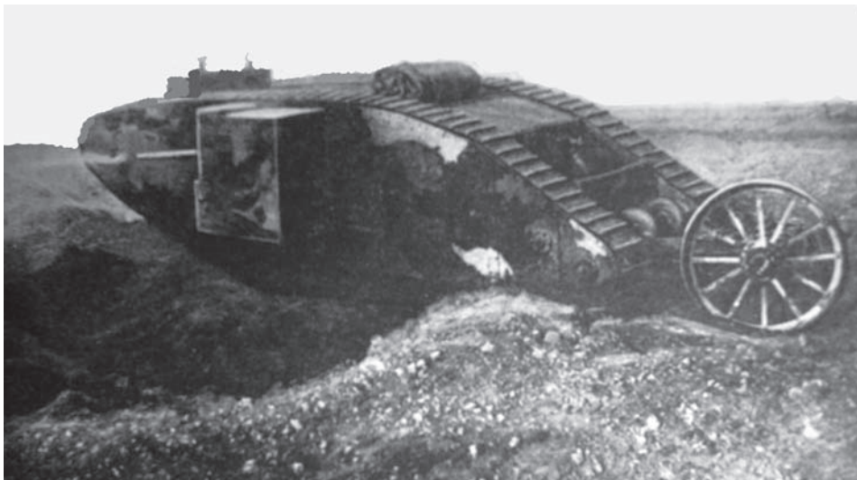
A "Male" Mark I tank in action on the Somme, 15 September 1916. Note the rear steering wheel – dispensed with in later Marks.
